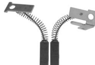
140161 Brush Set Replacing: ulb105, 60600780 Servicing: A115, A133, 23983, 23983A, 23984A, 23985A, 23986A, 23996A, 23996D, 23997A, 23998A, 23999A, 23999B, 24020A, 24023A 14 V, Length 20.00/22.00, Lead length 37.50, Height 7.00, Thickness 4.00
