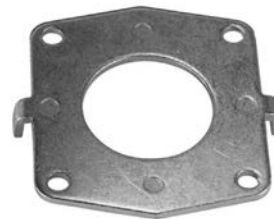
232059 Bearing Plate Servicing: A115I, 063341658000, 063377002010, 063377423010, 063377424010, 063377425010, 63320289, 63320511, 63321200, 63321204 ID 28.00, OD 57.10, Thickness 2.00, No./ mount. holes 4, Gasket w/o
