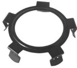
232736 Bearing Retainer Servicing: CS130 ID 44.50, OD 69.20 Bearing plate for 6303. Bearing used w/ D.E bracket.
