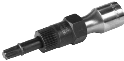
210909 Combi Tool Servicing: Valeo Alternators 33 teeth combitool for disassembly and assembly of free wheel pulley. Torx 50x110 mm, w/ 1/2" socket and 22 mm hexagon.
