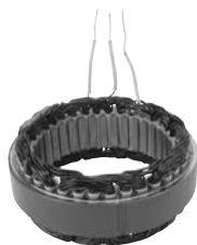
130105 Stator Replacing: 16.350.083 28 V, 45 Amp, ID 89.45, OD 125.00, OD 2 117.00, Height 23.55, Terminals 3
