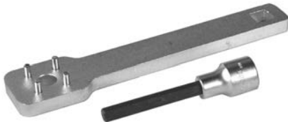
210873 Combi Tool Servicing: Magneti Marelli For removing and installing of rubber clutch pulley. 200 mm spec. tool + 8x100 mm allen wrench w/ 1/2" socket.
