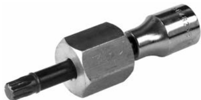
210877 Combi Tool Servicing: Bosch For removing and installing of rubber clutch pulley. XZN 10x112 mm w/ 1/2" socket and 30/28 mm hexagon.
