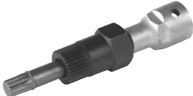
210843 Combi Tool Servicing: Bosch Alternators 33 teeth combi tool for the disassembly and assembly of the free wheel pulley. XZN 10x110 mm, w/ 1/2" socket and 22 mm hexagon.
