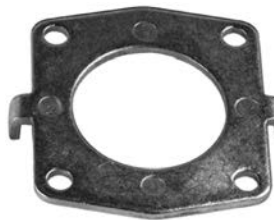
232060 Bearing Plate Servicing: A115I, 063377009010, 63321200, 63321233, 63321234, 63321235, 63321270, 63321280, 63321281, 63321286, 63321292, 63321300 ID 28.00, OD 48.90, Thickness 2.00, No./ mount. holes 4
