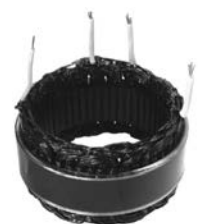
134731 Stator Replacing: 16.350.085, 16.350.073 28 V, 95 Amp, ID 125.33, OD 166.00, OD 2 157.50, Height 44.05, Terminals 4
