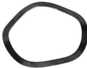
136296 Spring ID 33.00, OD 39.10, Thickness 0.50, Material Steel For 6203 bearing.
