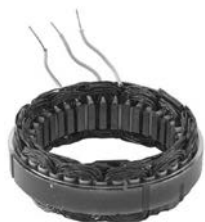
131457 Stator Replacing: 16.350.043 28 V, 27 Amp, ID 88.90, OD 125.00, Height 17.90, Terminals 3
