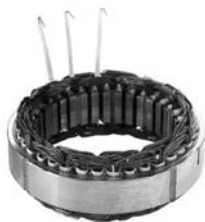
130106 Stator Replacing: 16.350.090 28 V, 35 Amp, ID 89.40, OD 125.00, OD 2 118.00, Height 23.50, Terminals 3
