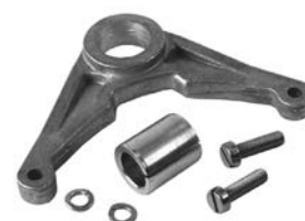
230281 Support Bracket Replacing: 16.905.302 Servicing: 11.201.055, 11.201.070, 11.201.071, 11.201.075, 11.201.304, 11.201.306, 11.201.324, 11.201.325, 11.201.326, 11.201.327 Mount hole 5.55, Mount. hole 2 5.55, ID 12.25, Thickness 7.80, Dist. mount. holes 91.95
