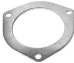
232763 Bearing Retainer Plate Replacing: 10467271 Servicing: 21SI, 22SI, 3G series, 1117839, 1117880, 1117885, 1117886, 1117887, 1117890, 1117891, 1117892, 1117894, 1117895 ID 53.55, ID/ threaded hole 5.90, OD 75.00, Thickness 2.00, No./ mount. holes 3
