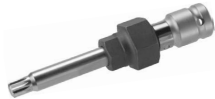
211081 Combi Tool Servicing: Valeo For removing and installing of rubber clutch pulley. XZN 10x128 mm w/ 1/2" socket and 28/19 mm hexagon.
