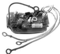
131903 Regulator Replacing: d693, 1969110, 1892824, 10498824, 10457127 Servicing: 25SI, 1117069, 1117226, 1117229, 1117236, 1117238, 1117239, 1117243, 1117248, 1117249, 1117250, 1117253, 1117254 27.5 V setting, Dist. mount. holes 49.75, Regulator type Electronic Neg. ground.
