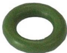
250439 O-ring Replacing: 100400400 Servicing: Alfa Romeo, Audi, Vw, Citroen, Peugeot, Fiat, Ford, Honda, Acura, Hyundai, Mazda, Mercedes, Misubishi, Opel, Vauxhall ID 4.47, Thickness 1.78, Material HNBR
