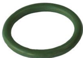
250110 O-ring ID 18.50, Thickness 2.50, Material Nioprene
