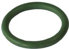
250110 O-ring ID 18.50, Thickness 2.50, Material Nioprene
