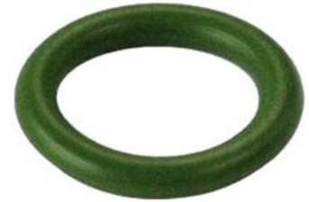
250489 O-ring Servicing: Nissan, Calsonic ID 10.90, Thickness 2.43, Material HNBR
