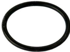
250656 O-ring ID 23.00, Thickness 2.00, Material HNBR
