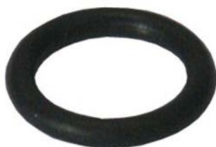
251581 O-ring ID 12.00, Thickness 2.50, Material Nioprene
