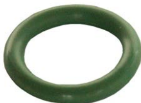
252164 O-ring ID 12.37, Thickness 2.62, Material HNBR
