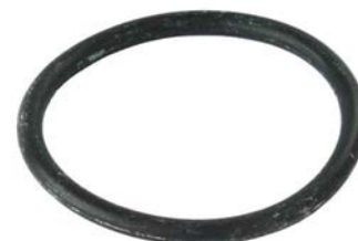
250156 O-ring Servicing: 047200-9432 ID 34.00, Thickness 3.00, Material Nioprene
