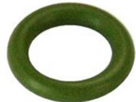
250460 O-ring Servicing: BMW, Mazda, Mitsubishi, Renault, Suzuki ID 6.07, Thickness 1.63, Material HNBR
