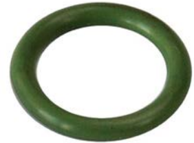
250457 O-ring Servicing: Alfa Romeo, Mitsubishi, Opel, Vauxhall ID 13.95, Thickness 2.62, Material HNBR
