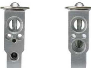
260541 Expansion Valve Replacing: 1638300084 Servicing: Mercedes-Benz A: 84.95 B: 25.85 C: 42.50 mm
