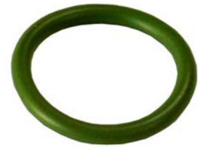
250459 O-ring Servicing: Alfa Romeo, Fiat, Honda, Acura, Hyundai, Mazda, Mercedes, Mitsubishi, Opel, Vauxhall, Renault, Toyota ID 18.72, Thickness 2.62, Material HNBR
