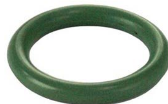
250154 O-ring Servicing: 047200-8602 ID 14.50, Thickness 2.50, Material Nioprene
