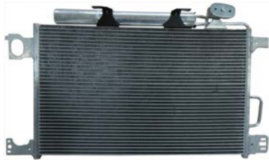
260422 Condenser Replacing: 2035002154 Servicing: Mercedes-Benz Dryer w/ A: 382.00 B: 628.00 C: 20.00 mm
