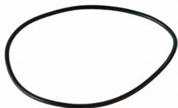
250003 O-ring Servicing: 047200-8545, 047200-8602, 447200-0100, 447200-0101, 447200-0102, 447200-0103, 447200-0104, 447200-3083, 447200-3234 ID 108.00, Thickness 3.00, Material Nioprene
