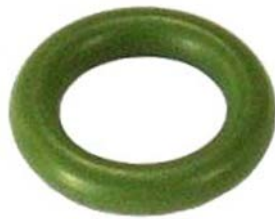
250487 O-ring Replacing: 92470-N8210 Servicing: Hyundai, Nissan, Calsonic ID 6.88, Thickness 1.77, Material HNBR
