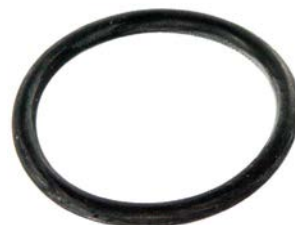
252601 O-ring ID 29.20, Thickness 3.00, Material Rubber
