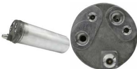
260117 Dryer Replacing: 46745058 Servicing: Fiat A: 60.00 B: 188.00 mm
