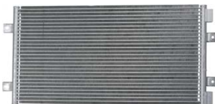
260028 Condenser Replacing: 46799862 Servicing: Fiat Dryer w/o A: 316.00 B: 608.00 C: 20.00 mm
