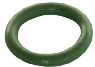
252164 O-ring ID 12.37, Thickness 2.62, Material HNBR
