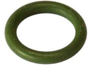
250491 O-ring Servicing: Nissan, Calsonic ID 11.00, Thickness 2.40, Material HNBR
