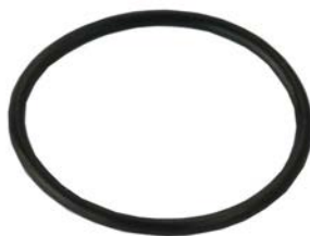
250604 O-ring ID 29.50, Thickness 2.00, Material Nioprene
