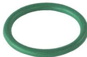
250082 O-ring Servicing: 047200-2920, 047200-3523, 047200-3792, 047200-4033, 047200-6370, 047200-6480, 047200-7030, 047200-7480, 047200-7501 ID 24.50, Thickness 3.00, Material HNBR
