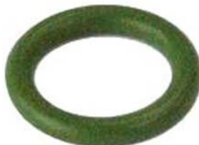
250438 O-ring Replacing: D7RS7, D7RSA7 Servicing: Fiat, Honda, Acura, Mazda, Mitsubishi, Renault, Suzuki, Toyota ID 7.00, Thickness 1.50, Material HNBR
