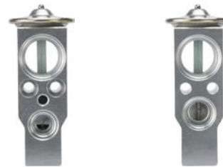
260530 Expansion Valve Replacing: 6461K0 Servicing: Citroen, Peugeot A: 84.30 B: 25.55 C: 32.55 mm
